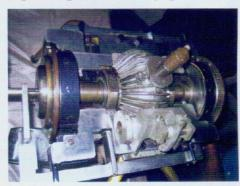
to petrol to Diesel! The new engine design also guarantees a reduction in wear and vibrations through the elimination of piston slap which will mean a smoother and quieter drive.
